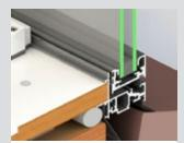
Integrating the frame with the reveal delivers a minimalist design aesthetic and optimal viewing plane to the outdoors.
