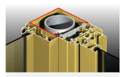
There are numerous snap couplers that allows us to join window to window or window to door. The illustration above shows the  $90^\circ$  corner coupler designed to wrap around support posts. No unsightly rivets or screws required.
